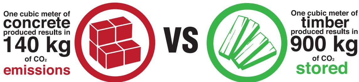
The net CO<sub>2</sub> emissions of different building materials vary greatly during their life cycle. Whereas wood-based construction materials - such as timber, plywood, particle boards and hardboards - absorb carbon, mineral-based construction materials - like gypsum board, limestone and red bricks - and metal-based construction materials - such as steel plates and rolls, steel I-beams and aluminum façade elements - cause significant carbon emissions during their life cycle.
